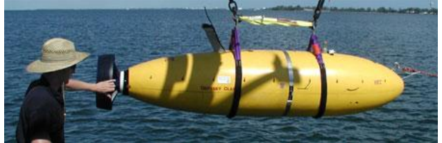
Fig. 1. Caribou AUV. Our experiments used an Odyssey-III class vehicle equipped with DVL/LBL/GPS and INS. The primary payload of Caribou was a synthetic aperture sonar (SAS), not pictured. While we did not use data from the SAS, our algorithms were designed to cope with the interference it caused.
